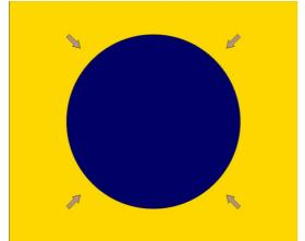
Allow the paint to dry sufficiently before removing the paint mask. While removing it is important to ensure the four arrows of the "A" mask are retained on the model. These will act as registration marks for the application of the "B" mask later.
